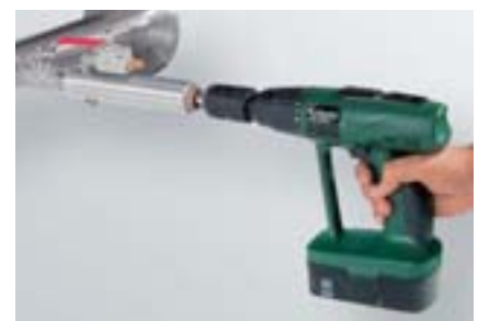
• Drilling under pressure
