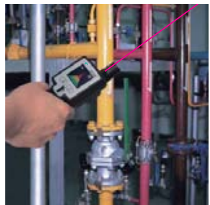
The integrated laser facilitates the detection of leaks.
